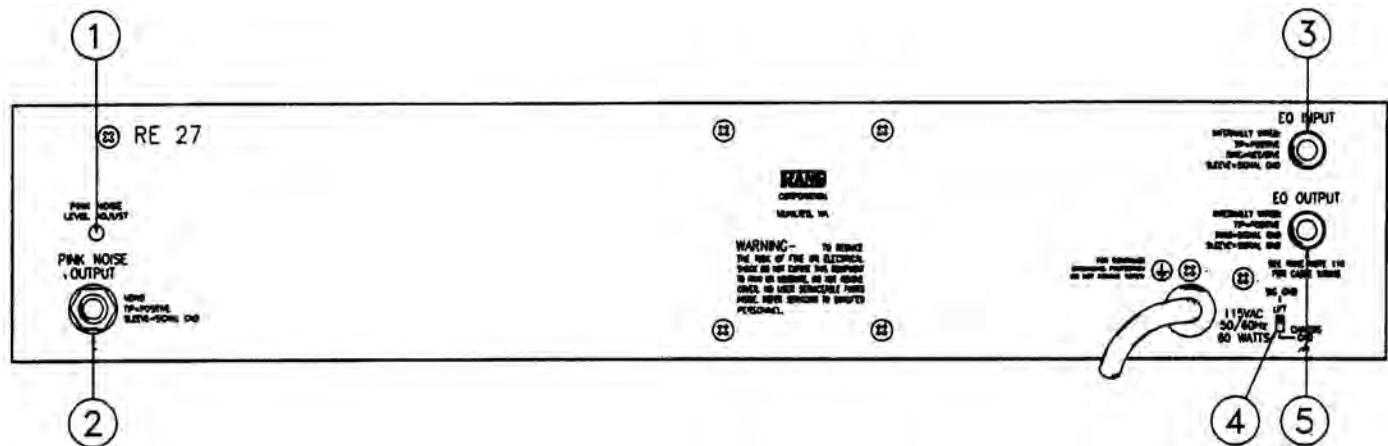
1. PINK NOISE LEVEL ADJUST: Use a 1/8" screwdriver to adjust the output from the Pink Noise generator from 0 to 1.2 volts (-4 dBu) to match the input level requirements of the mixer or other equipment.
