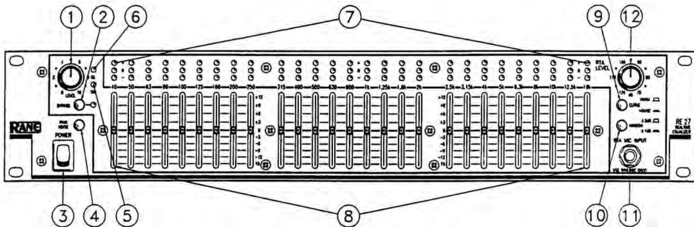
1. EQ LEVEL CONTROL: This controls level through the equalizer section and provides up to 6 dB overall gain. Turn this control down if the overload LED lights up.
