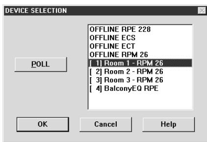
The DEVICE SELECTION window displays the list of available RW 232 units, including the OFFLINE versions of each RW 232 product. The OFFLINE versions allow you to operate the software just as if you had an actual unit hooked up.
