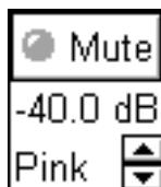
The signal Generators default to a Muted state when new DSP Programs containing Generators are requested. Click Mute to unmute the Generator. Click the up or down arrows to adjust the Generator's Level in  $\frac{1}{2}$  dB steps. The maximum attenuation is 40 dB. The Generator levels are calibrated in dBFS, i.e. at 0dB the Generator is sending a full scale digital signal to the D/As.
