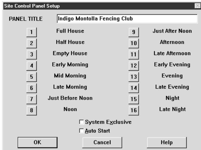
RaneWare's Site Control Panel (shown at right) is a sound system re-configuration screen. It works by telling *all* connected Rane RW 232 devices to switch immediately to a designated memory that you have programmed in each unit. Use the Site Control Panel Setup window (above) to customize the Site Control Panel's Title and Memory names.
