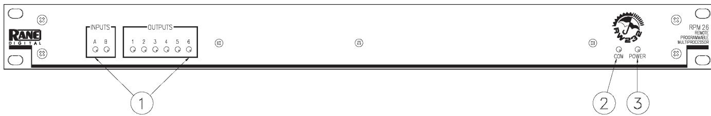
**1. Signal/Overload.** These multi-color LEDs indicate the presence of a significant audio Signal (green) or Overload conditions (red). Both Input and Output indicators are provided for signal flow verification without a computer. The Inputs' Signal LEDs are driven from an analog comparator circuit prior to the input level control. All other LEDs are controlled from the microprocessor.
