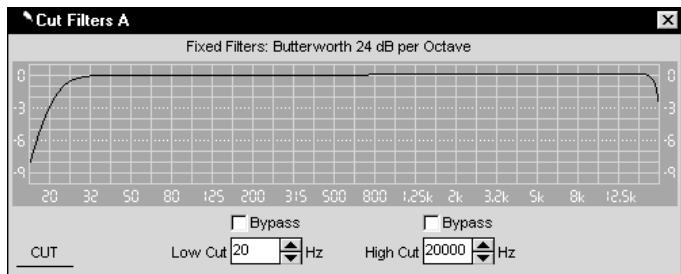
Like all detail windows, the name of the window is displayed at the top. The edit boxes at the bottom of the window show the current Low Cut and High Cut frequency settings in Hertz. To edit the current values, click the up or down arrows, or click in the edit box to display the cursor and type a new value. The High and Low Cut filters are fixed Butterworth, 24 dB/Oct. (4<sup>th</sup> order) filters.
