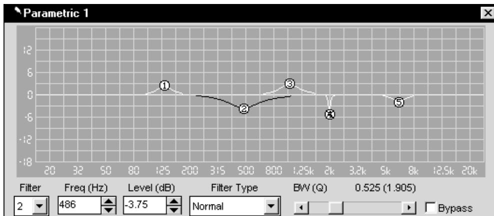
filter. (See the EXTENDED PARAMETRIC section below for additional filter types such as Linkwitz-Riley, Bessel and Butterworth filters.) Those systems that require constant directivity horn equalization can use the High Shelf PEQ Filter Type in combination with other PEQ filters to achieve the appropriate EQ for the combination of horn and compression driver you are using. For optimum frequency response, use an analyzer to achieve the best possible horn EQ compensation.
