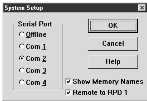
The Serial Port radio buttons on the left tell the computer which Com port is being used to “speak” to the connected RW 232 unit(s). The Offline radio button permits use of the software without connecting a unit. To operate an RW 232 unit, you must select the Com (serial) port that is physically connected to the unit. This screen is also displayed the first time you start RaneWare or after erasing the RW232.INI file from your Windows directory.
