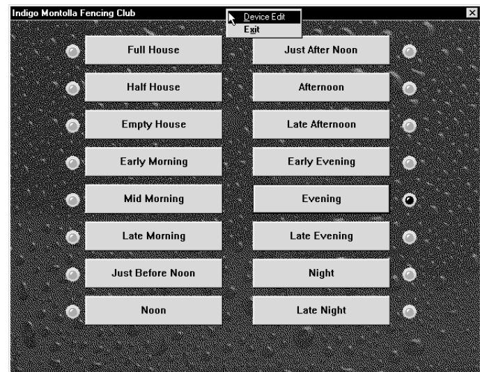
The Site Control Panel is RaneWare's sound system re-configuration screen. Depending upon how you set up the control panel (using Site Control Panel Setup), up to 16 buttons can be displayed and each can have a unique name representing a particular sound system configuration.
