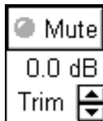
input and send the same +20 dBu out. This +20 dBu is designed to be zero dB Full Scale (dBFS) at the A/D converter (i.e., maximum input to the A/D converter) when the Input Trim is set to 0.0dB. *Set the Input Trim so your nominal signal level lights the A/D meter indicator corresponding to your system's required headroom.*
