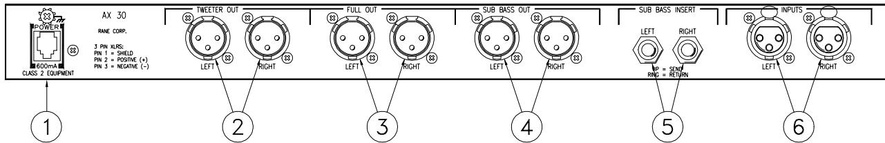
① **Remote power supply input:** This unit is supplied with a Rane RS 1 Remote AC Power Supply suitable for connection to this input jack. The power requirements call for an 18 VAC center-tapped transformer. *This is not a telephone jack. Never use a power supply other than the one supplied or a replacement approved by Rane.* Using any other type of supply may damage the unit and void the warranty.
